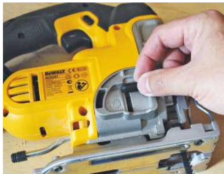
▲ On the right-hand side of the jigsaw is the adjustable blower lever
